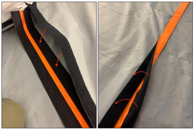
18. Fold the outer run of hook material up and over to sandwich the X-Series Floor in the orange portion of the joining strip.
