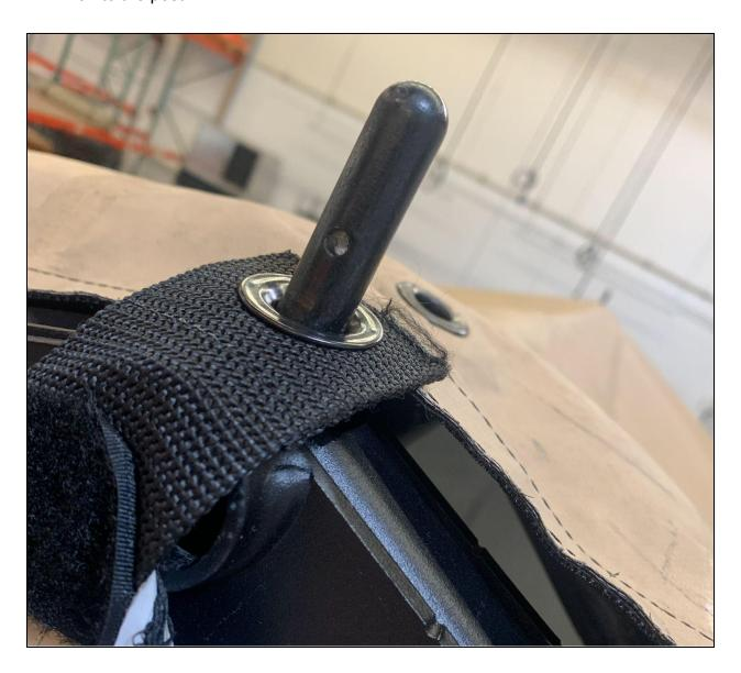
8. Pull the roof back on to the frame post and secure it with the pin.
